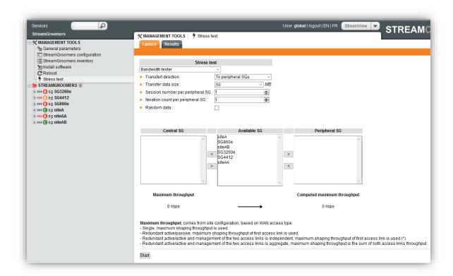
**WARNING**: This test is generating traffic up to the physical capacity of a link (either on the remote site or on the server side). Saturating the link will cause other traffic to be delayed or dropped. It is advisable to carry Stress test sessions when it will not harm critical traffic and usually out of traffic peak hours.
