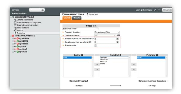
Note: It is advisable to request multiple sessions to multiple remote SG if the network is based on redundant links as load balancing algorithms will not work with a single connection.
